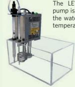
The LE13000 Thermo regulated pump is used to heat and recirculate the water that maintains a constant temperature in the tissue chamber.
